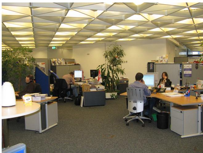
**Fig. 7** Open space with only a few free-standing barriers and with BGN = 47dB(A)
